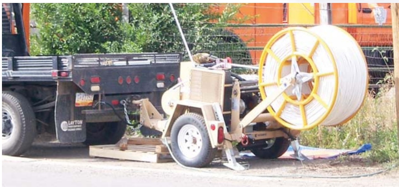
Built-in self-loading reel winder.
