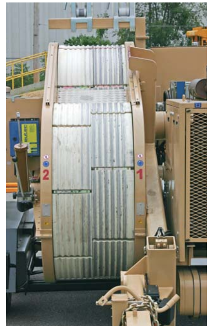
Interchangeable Nylon Sectors.
