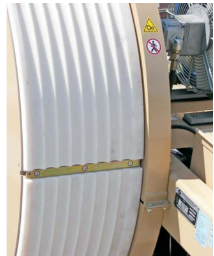
Interchangeable Nylon Sectors.
