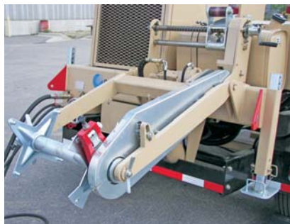
Built-in self-loading reel winder.
