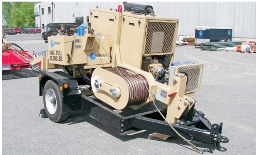
Bull-wheel grooves are manufactured of heat treated steel.
