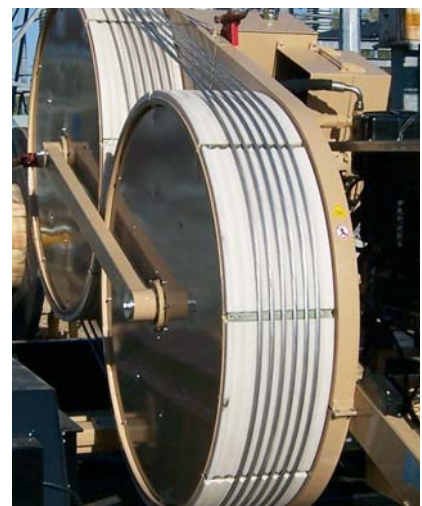
Interchangeable Nylon Sectors.
